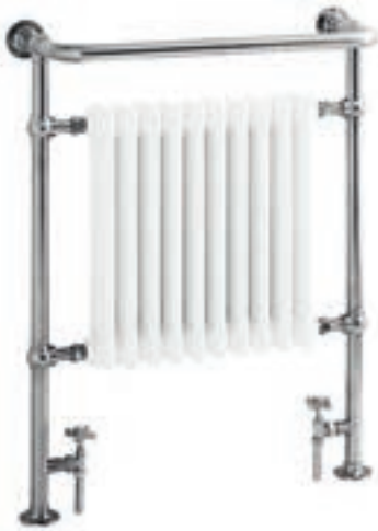
Clifton Height 940mm Width 734mm Valve centres 510mm Wall to valve centre 105mm Output 2340 Btu (686 watts) Chrome, White Bars AHC73 £650 Chrome, Black Bars AHC73B £675
