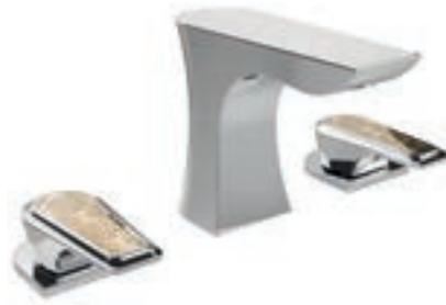
3 Taphole Basin Mixer Spout projection 95mm Full height 110mm Min. operating pressure 0.2 bar Valve: Quarter turn ceramic disc Lace Gold Inlay TLYCG06 £290
