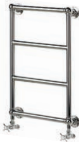
Portland Wall Mounted Height 740mm Width 475mm Valve centres 400mm Wall to valve centre 80mm Output 475 Btu (139 watts) Chrome AHC94 £375
