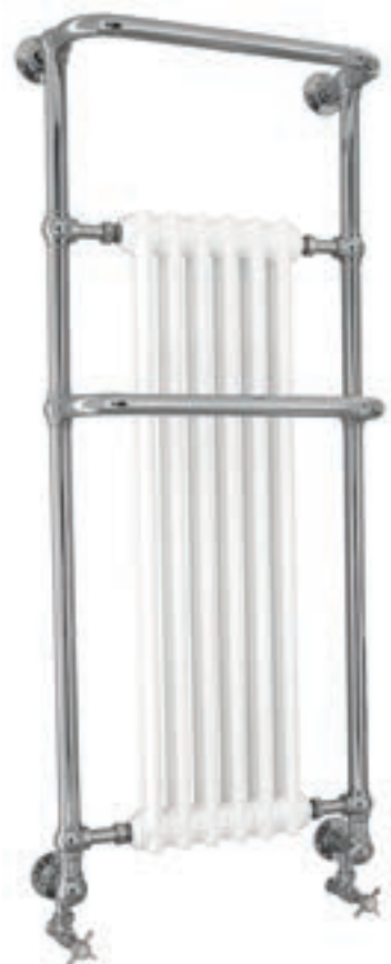
Cabot Wall Hung Height 1355 (exc. Valves)mm Width 574mm Valve centres 500mm Wall to valve centre 55mm Output 2167 Btu (635 watts) Chrome AHC102 £775
