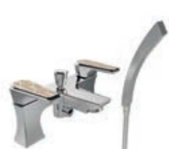
Bath Shower Mixer Spout projection 105mm Full height 106mm Min. operating pressure 0.2 bar Valve: Quarter turn ceramic disc Inlet centre 180mm Hose length 1750mm Lace Gold Inlay TLYCG02 £390
